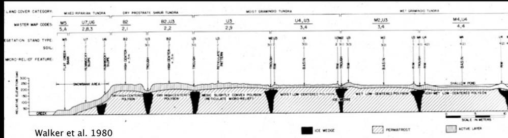
Schematic of an actual 300-m trench through ice-wedge polygons showing the areas of massive ground ice (blue)
