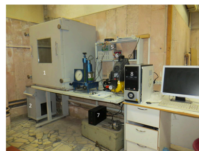
Triaxial shear test equipment
