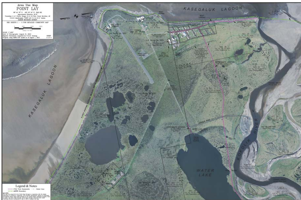
Figure 10. Village of Point Lay and vicinity. Ice-wedge polygons occur nearly everywhere in lake basins and remnant surfaces of various age. Roads passing through the lake basins block the natural drainage patterns causing local flooding. The village is on a yedoma deposit with large ice wedges that are degrading rapidly and threatening the foundations of many of the houses (Fig. 7C) and the village’s buried utility system. The water lake near the bottom of the image was the village water supply and drained into the Kokolik River in 2016 due to thermal erosion of ice wedges in the lake shore.
