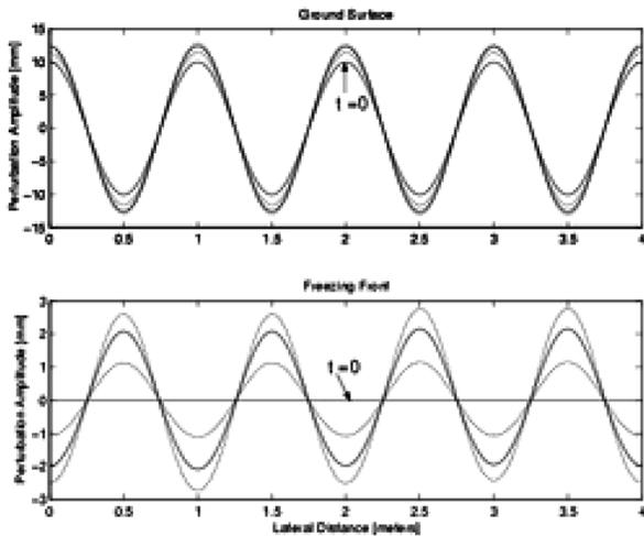
Figure 3. Time series showing the perturbation amplitudes for both the ground surface and freezing fronts. Amplitudes increase with time and each curve is for  $\Delta t = 7.3$  days. The freezing front is initially flat and the ground surface amplitude is initially 1 cm. Amplitudes are measured relative to their mean location, so the above figure does not show the increase in freezing depth that is occurring.
