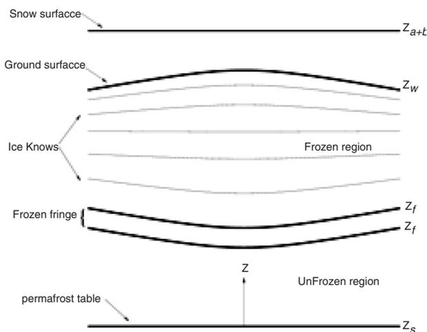
Figure 2. Schematic of soil undergoing top-down freezing on which the DFH model is based. Ice lenses exist in the frozen region and permafrost underlies the active layer.
