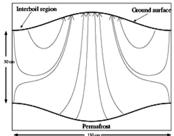
Figure 5. Particle trajectories over several hundred years of differential heaving and soil creep. Soil particles move downward in the inter-boil region and upward beneath the center of the frost boil.
