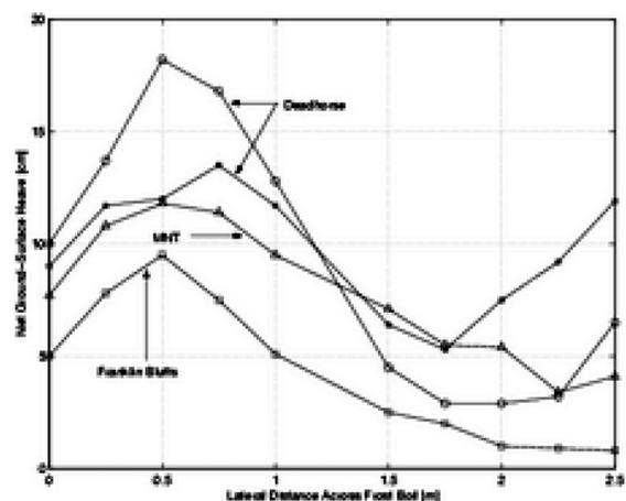
Figure 1. Net ground-surface heave recorded in spring from the heave meters. Errors in the measurements are  $\pm 1$  mm.
