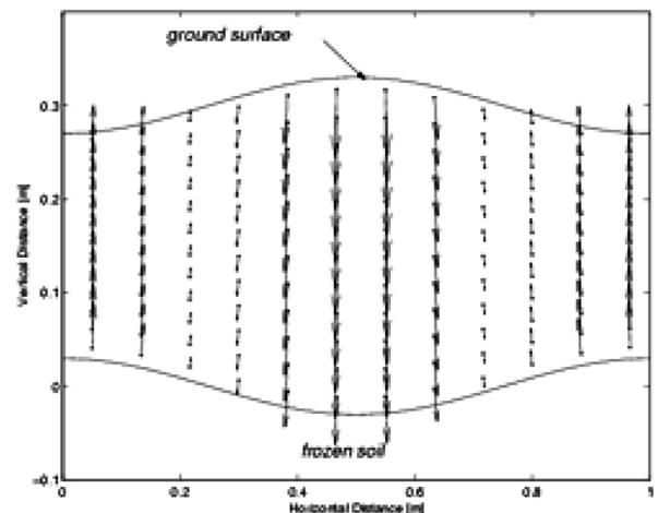
Figure 6. Particle trajectories of unfrozen soil using a viscous-relaxation model to describe soil creep. The arrows indicate direction and relative magnitude of soil particles.
