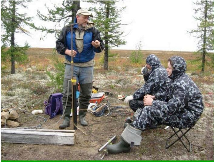
Temperature measurement in bore-hole
