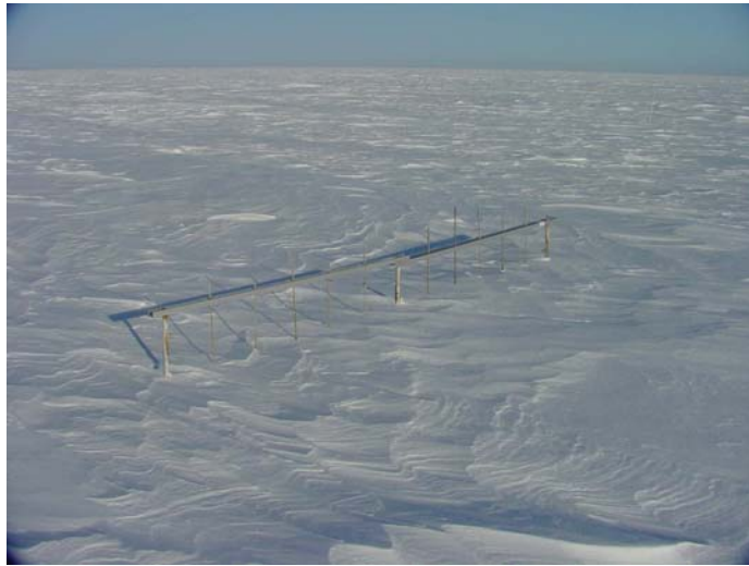
Photo 5. Heave-meter at Franklin Bluff moist grid. Photo by M. K. Raynolds
