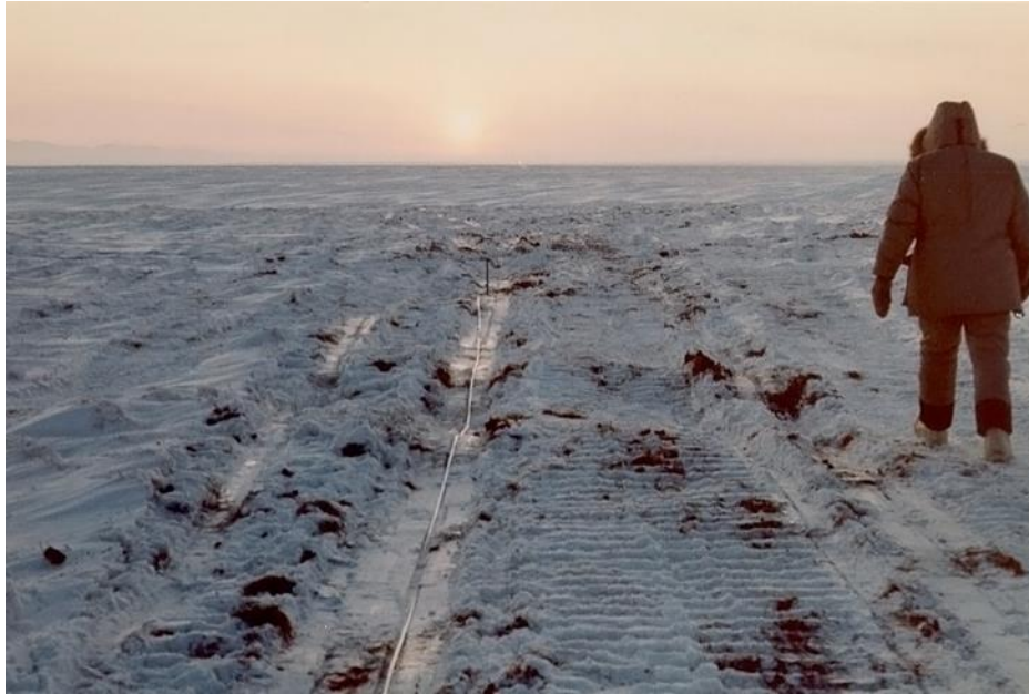
Figure 14. Trail made by D-7 Caterpillar tractors and ski-mounted trailers in March 1984. This site was still highly disturbed in 1994. 74 By 2018 the trail here had subsided into a large pond due to melting of ice wedges. Based on the amount of bare ground exposed, it is clear that there was insufficient snow to protect the tundra. 75
