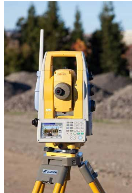
Figure 2.6. Topcon IS-3 Imaging Station and Laser Scanner. Photo: Topcon.
