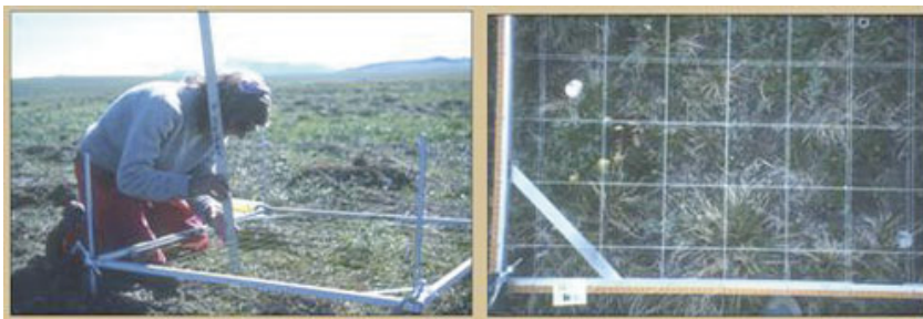
Figure 2: (Left) Point quadrat used in sampling. The vertical legs are positioned in metal guides that are nailed into the tundra. The frame can be repositioned exactly in successive sampling years by leveling the frame, clamping it securely, and aligning it to a set of metal registration points that are nailed into the tundra at 4 grid points (black «X» in the species plots in Figure 3). (Right) Two parallel grids of monofilament line, one above the other, are spaced 2 cm apart. Aligning the intersection points in both grids permits unambiguous identification of points in the plant canopy. We recorded the species at the top and bottom of the plant canopy at each point and the distance from the bottom monofilament line to the top and bottom species.
