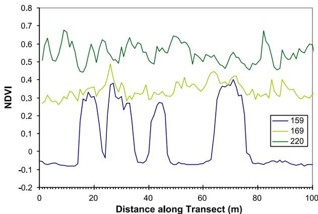
Fig. 2. Optical sampling from the tram system shows the dynamics of NDVI in both time and space. The distance axis is the position along the tram transect, and each line represents the NDVI values measured at every meter along the transect for the day of year of 2001 given in the legend. Day 159 (June 8) was very early in the season, before the snow fully melted, day 169 (June 18) was one of the first completely snow-free days, and day 220 (August 8) was near the seasonal peak growth.
