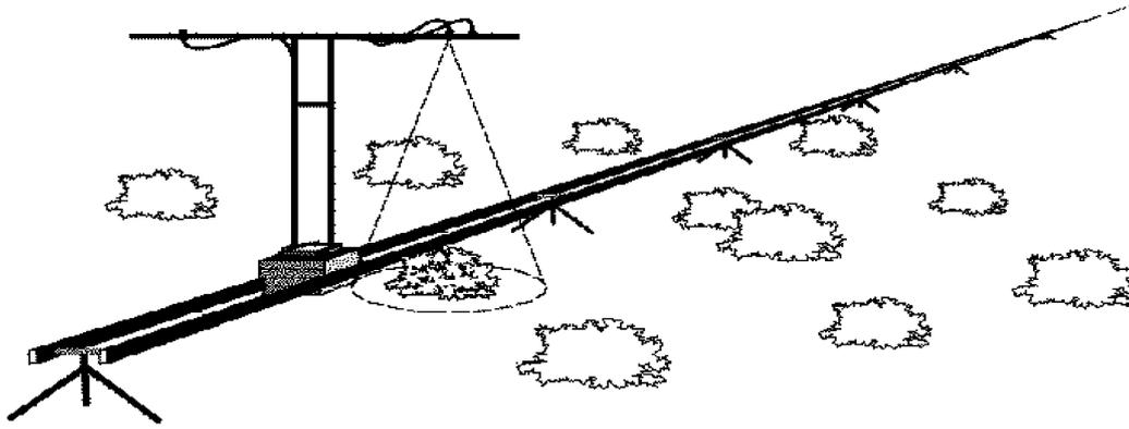
Fig. 1. A graphic display of key elements of the tram system used in the Barrow study. Tracks were leveled and supported above the ground by tripods. A cart ran along the tracks carrying the spectroradiometer. Two fiber-optic heads for the spectroradiometer were mounted on a tower attached to the cart with one head looking upward and the other looking downward at an area next to the tracks. The cart was stopped at every meter along the transect to collect a measurement.
