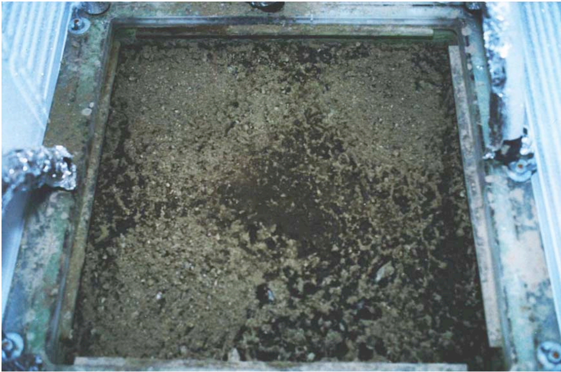
Figure 9. Photograph of four frost boils made prominent both by soil surface heave and sorting of stone. The center-to-center spacing of about 28 cm is in agreement with the model predictions of the most likely pattern to form at a 10-cm depth of freezing. The interboil region appears darker due to greater surface ice.
