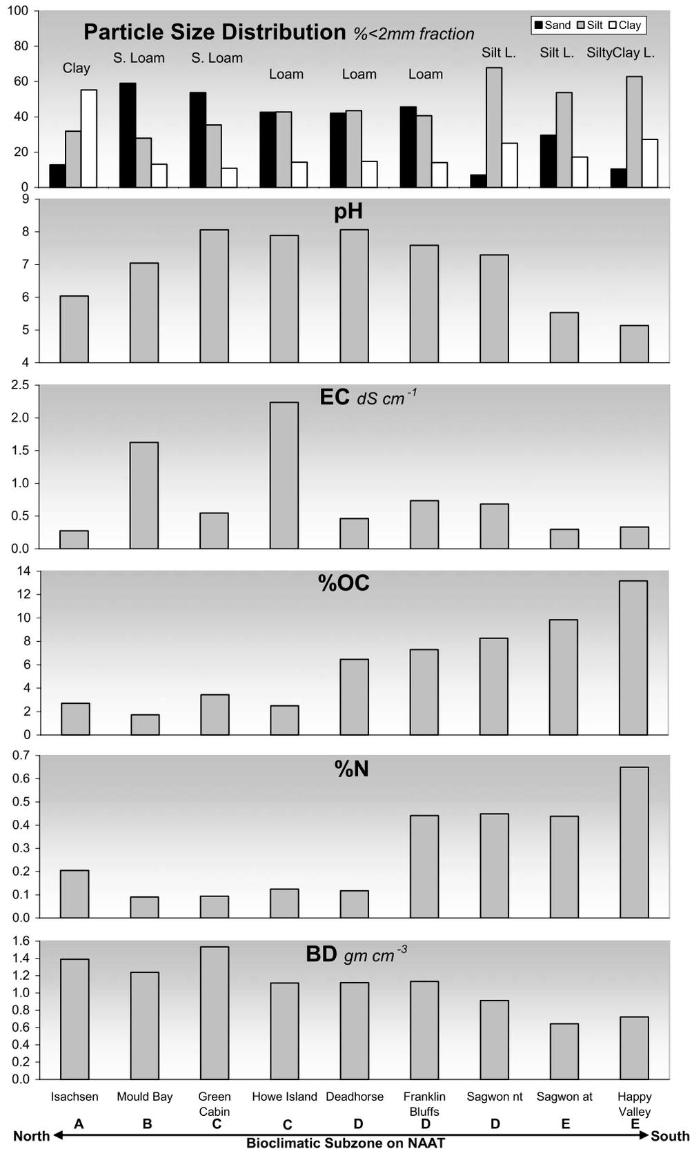
**Figure 2.** Selected average soil properties for profiles (to 1 m depth) of the zonal vegetation sites along the North American Arctic Transect (NAAT) with bioclimatic subzones according to Walker et al. [2005]. Averages are weighted sum of properties using relative horizons thicknesses as identified from the soil pit exposures to 1 m [Michaelson et al., 1996].
