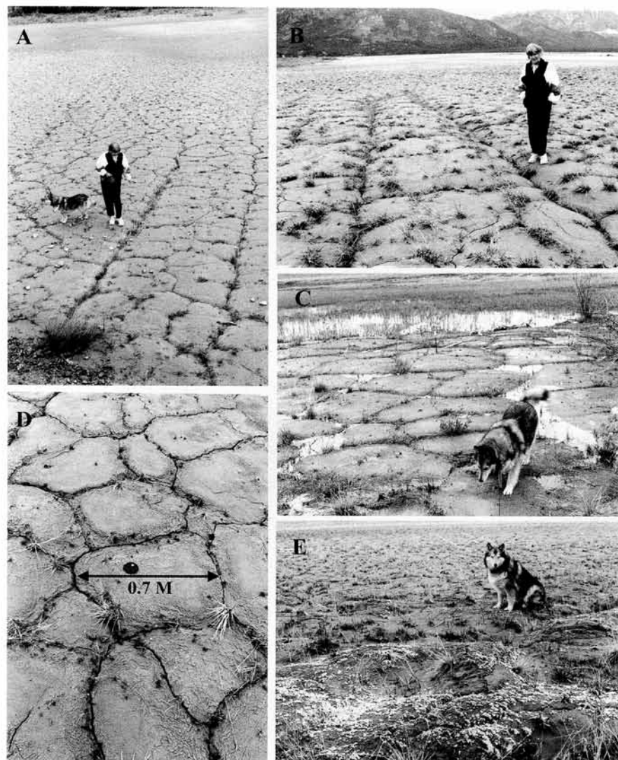
Figure 4.38 Thermal and desiccation cracking creating polygonal patterns in saturated, fine-grained soil deposited by Slims River where it empties into Kluane Lake at Mile 1028 on the Alaska Highway. Parts A and B show large parallel cracks spaced approximately 2 m apart with an inner array of polygonal cracks of spacing approximately 0.7 m, as shown in Parts C and D. The photo in Part E shows what appears to be a group of earth hummocks beginning to form. These are approximately 20 cm in height. Photographs taken August 1996.
