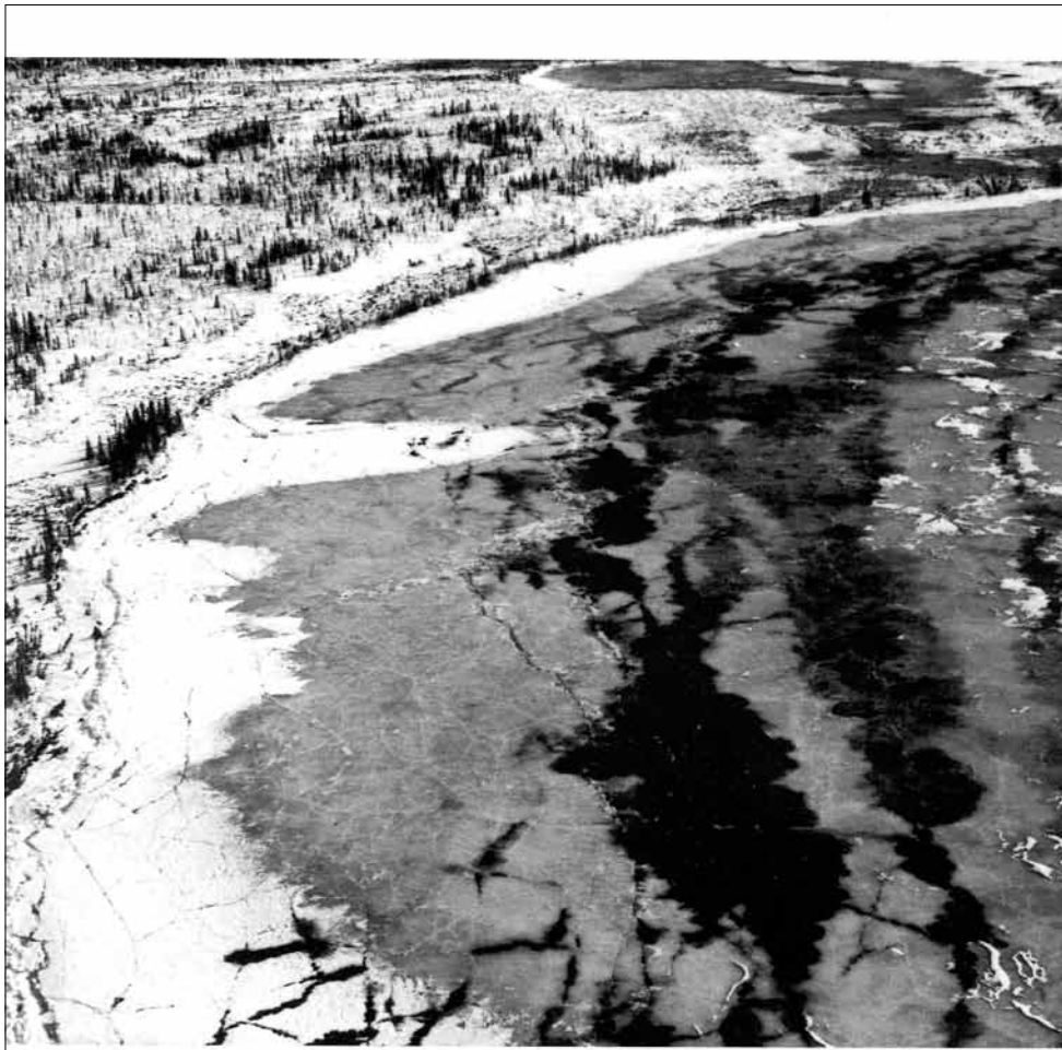
Figure 4.49 Mud thrown up by an earthquake darkens lake ice fractured by severe ground motion and sloshing of water below. Many lakes in the earthquake area showed such effects.
