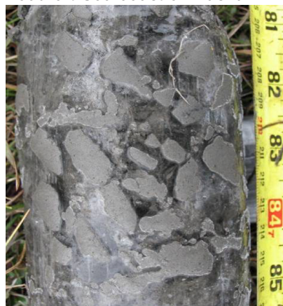
Figure 6. Ataxitic cryostructure in the upper permafrost, Beaufort Sea coast of Alaska.
