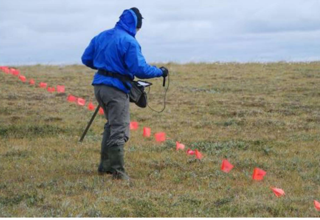
H.E. Epstein sampling NDVI using the PSII Spectrometer. Photo by D.A. Walker, 2007 A.V. Khomutov & M.O. Leibman measuring active-layer depth. Photo by G.V. Matyshek, 2007
