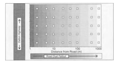
FIG. 2. Generalized diagram of sampling scheme at both sites. Study was designed to account for logarithmically distributed fallout of road dust (Everett 1980*a*). Replicate sample plots (represented as squares) were placed 20 m apart along eight 100-m parallel transects spaced at (approximately) logarithmically scaled distances from the road.
