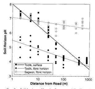
FIG. 3. Soil horizon pH at the Sagwon and Toolik study sites. Soil pH decreases to a normal level with increasing distance from the road at both sites. Each symbol represents a sample value for each plot at a site; symbol overlap may occur where plots have equal values. Samples were regressed against log of distance from the road; see Table 1 for regression line equations and significance of relationships.
